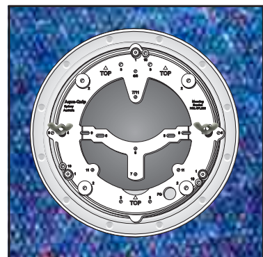
Place AQ Universal Mounting Bracket over the threads, tighten Wing Nuts to secure. Follow QC Instruction Manual to complete the installation.
